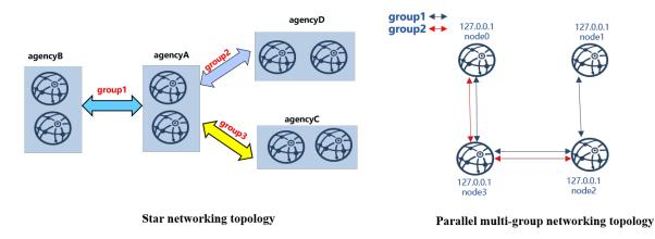
The following is a detailed description of how to deploy a eight-node star networking blockchain system and a four-node parallel multi-group networking blockchain.
