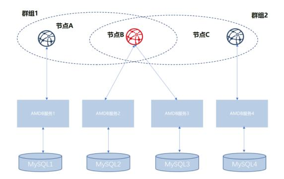
As shown in the above figure, NodeB belongs to multiple groups. The AMDB server and MySQL which are corresponded by the same node in different groups are separate. For distinguishing the same node in different groups, the nodes of A, B, and C are respectively represented with Group1\_A (NodeA in Group1, same as below), Group1\_B, Group2\_B, and Group2\_C.
